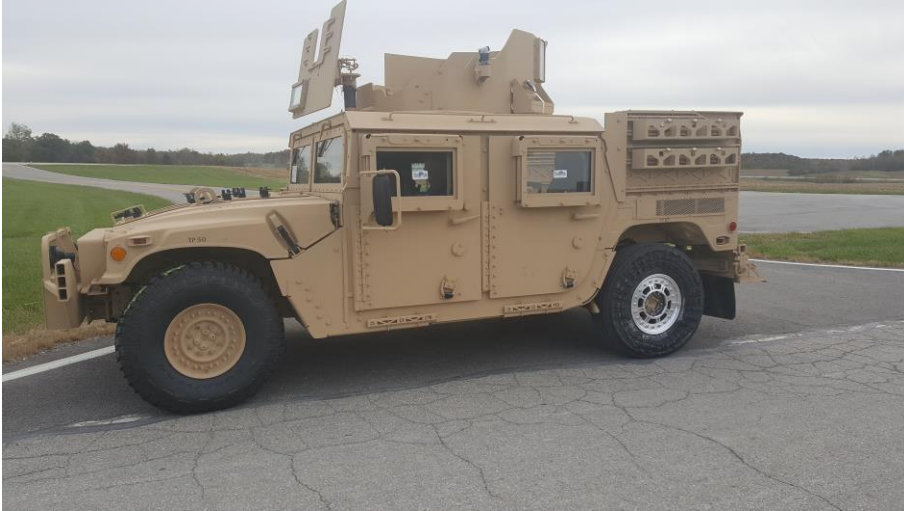
Figure 2: Test GMV vehicle provided by USSOCOM for AEG TRC testing(Fitted with AEG Pressure Zero Tire)
